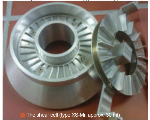
● Cut-away view of the shear cell (type XS-Mr, approx. 30 ml)
